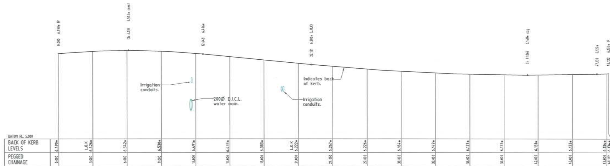
TURNOUT NE Scale 'A' - Horizontal Scale 'B' - Vertical "L.O.K." indicates lip of kerb level.
